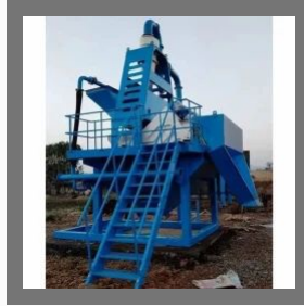
Semi-Automatic Sand Screening Machine
