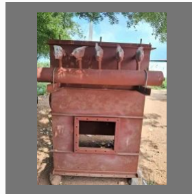
Bin Vent Dust Collector
